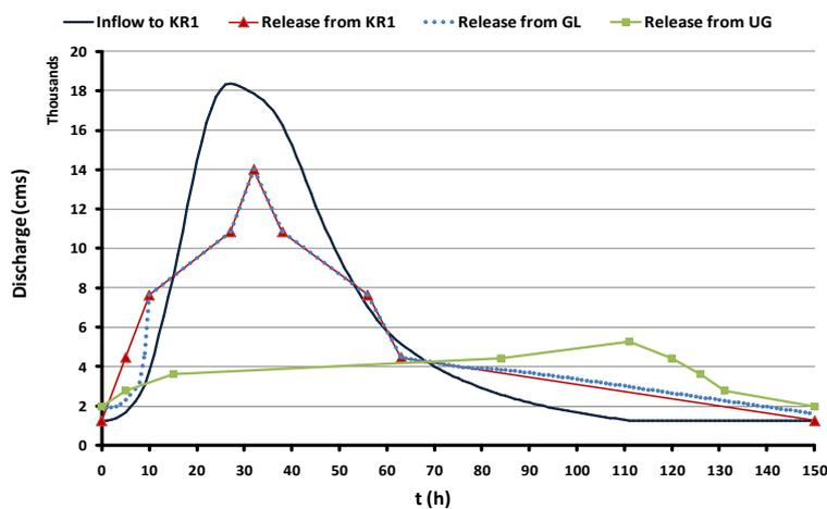
**Figure 6:** 10000-year inflow flood hydrograph to KR1 dam and optimal releases from KR1 and UG reservoirs and simulated releases from GL
