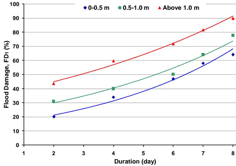
Figure 2: Flood damage function as a function of flow depth and its duration [42]
