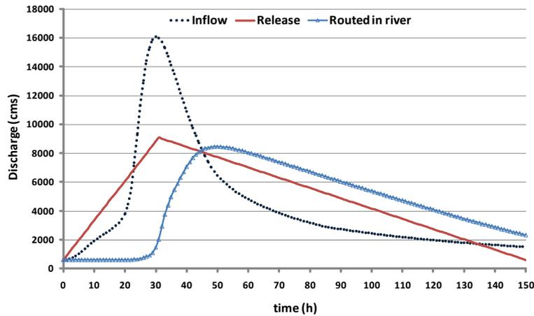
**Figure 5:** 10000-year inflow flood hydrograph compared to optimal reservoir release hydrograph at Dez dam and routed hydrograph at intersection with Karun river
