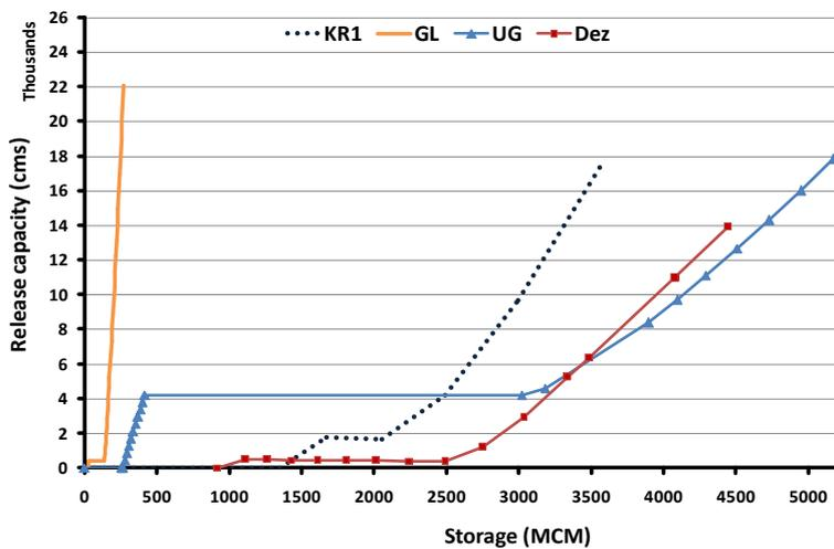
Figure 4: Outflow capacity curves of existing dams
