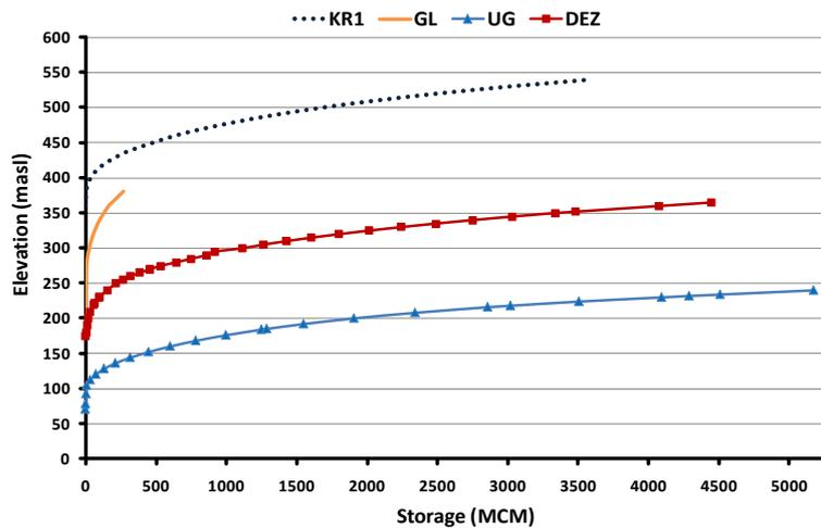
Figure 3: Storage vs. elevation curves of existing dams
