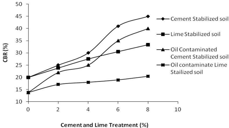
Fig. 10: Variation of CBR with Cement and lime Treatment for contaminated and uncontaminated stabilized soil
