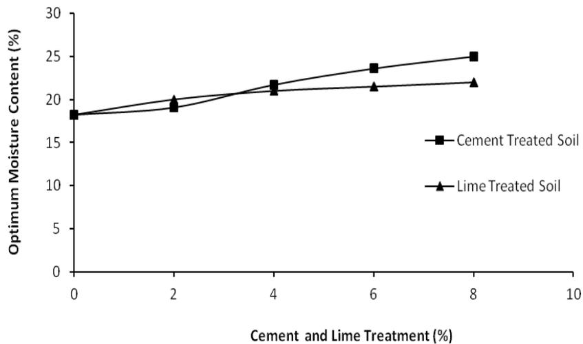
Fig. 3: Optimum moisture content of oil, cement and lime treated soil
