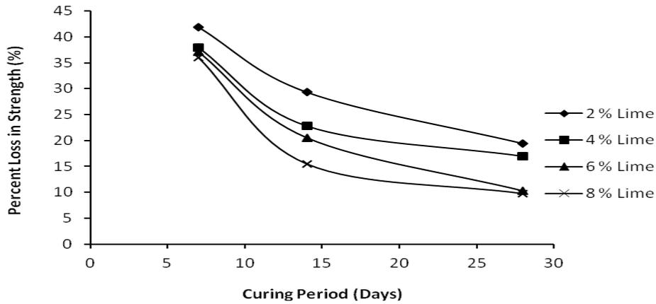
Fig. 8: Variation of PLS with Curing Period for Lime Stabilized Soil
