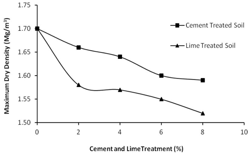
Fig. 2: Maximum dry density of oil, cement and lime treated soil
