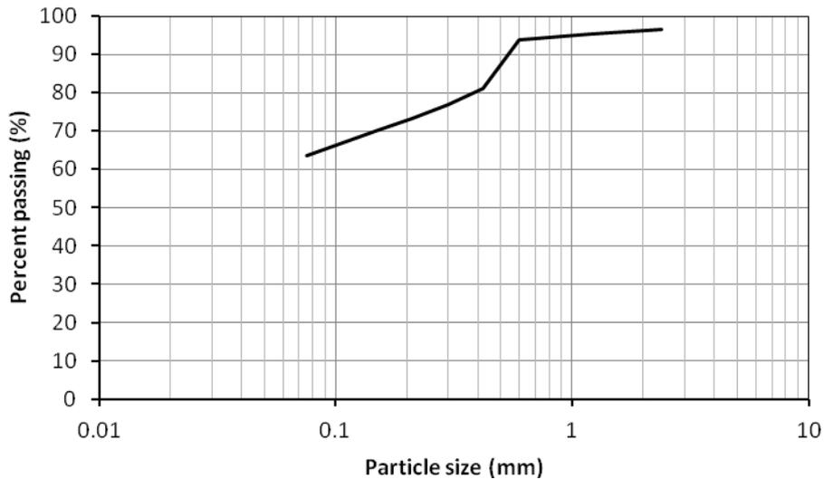
**Fig 1:** Particle size distribution of the laterite soil
