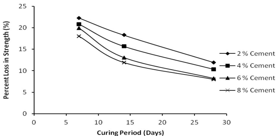
Fig. 7: Variation of PLS with Curing Period for Cement Stabilized Soil
