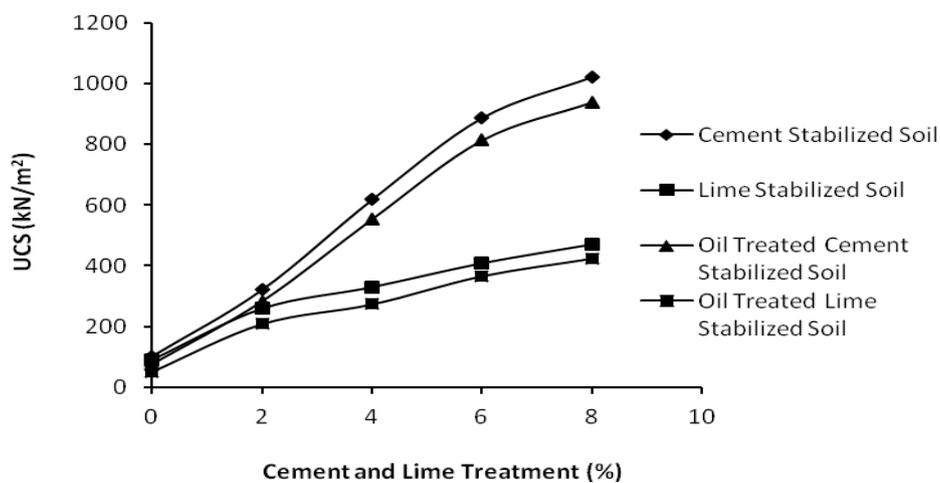
**Fig. 6:** Variation of UCS with Cement and lime Treatment for contaminated and uncontaminated stabilized soil (28 days curing)
