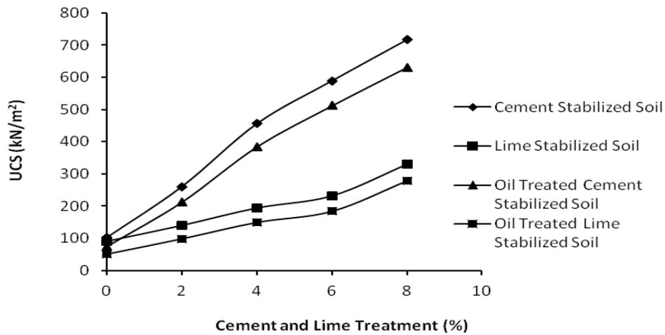
**Fig. 5:** Variation of UCS with Cement and lime Treatment for contaminated and uncontaminated stabilized soil (14 days curing)
