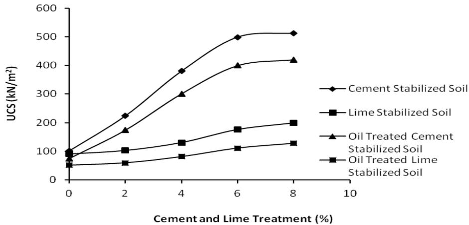
**Fig. 4:** Variation of UCS with Cement and lime Treatment for contaminated and uncontaminated stabilized soil (7 days curing)
