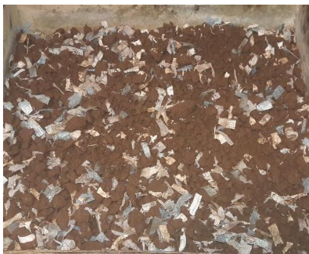
Figure 5. The mixture of soil and shredded face masks at their Optimum Moisture Content
