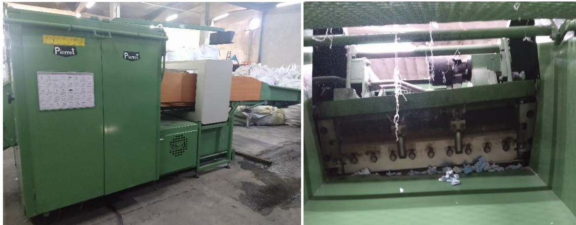
Figure 2: a) Guillotine used in the test crushing. b) Trial crushing of the face masks.
