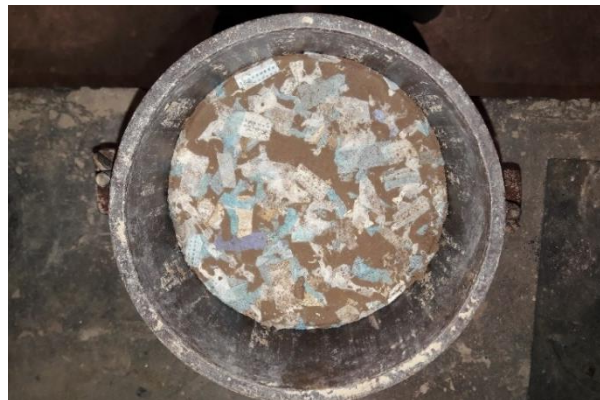
Figure 7: CBR test specimen surface with face masks content close to optimal
