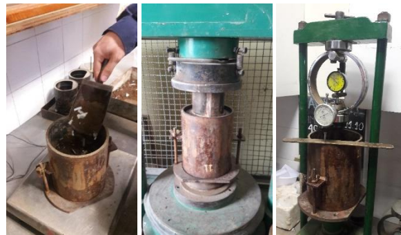
Figure 6: CBR test process with predetermined density molding
