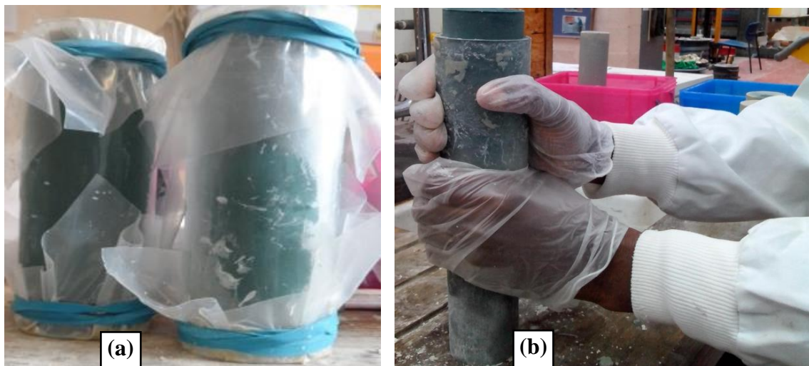
Figure 2 (a) samples cured in plastic moulds before extrusion, (b) sample extrusion
