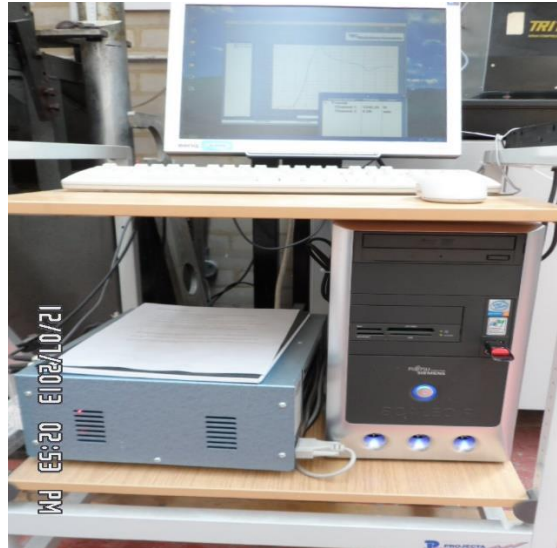
Figure 5 Data acquisition system attached to test apparatus
