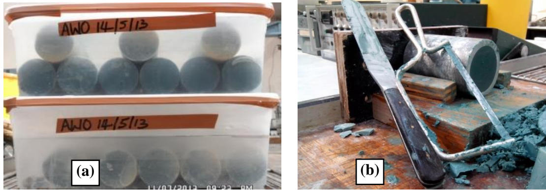
Figure 3 (a) samples curing under water; (b) cutting tools used for test specimen preparation
