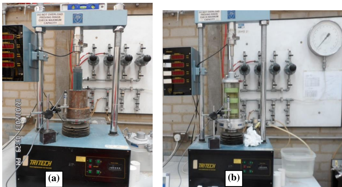
Figure 4 (a) UCS test load frame set-up, (b) triaxial test apparatus set-up
