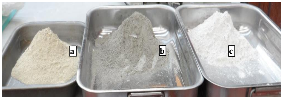
Figure 1 Mix materials: (a) Na-bentonite clay (b) PC (c) GGBS
