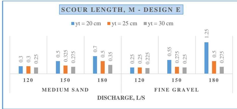
**Figure 13** Scour Length for Design E of Floor Jets with different Discharges, Tail Depths and Bed Materials
