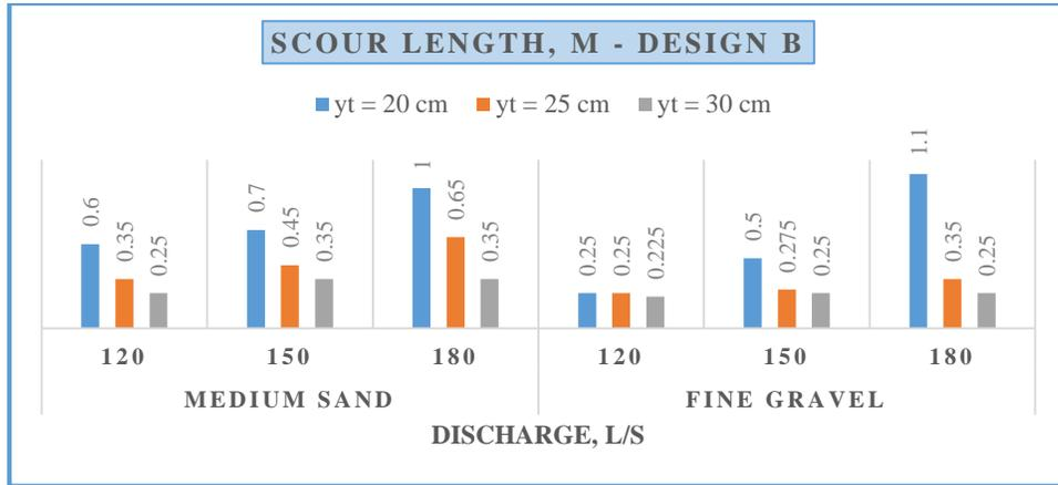
**Figure 10** Scour Length for Design B of Floor Jets with different Discharges, Tail Depths and Bed Materials
