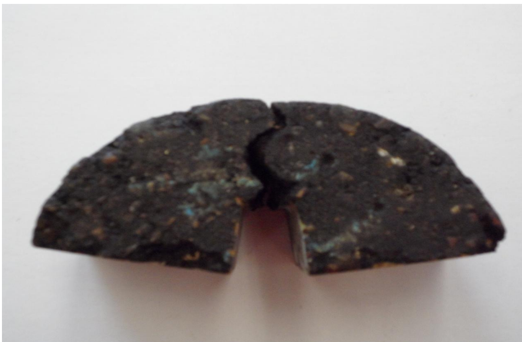
Figure 9: Crack Propagation at Test Temperature 20C°.
