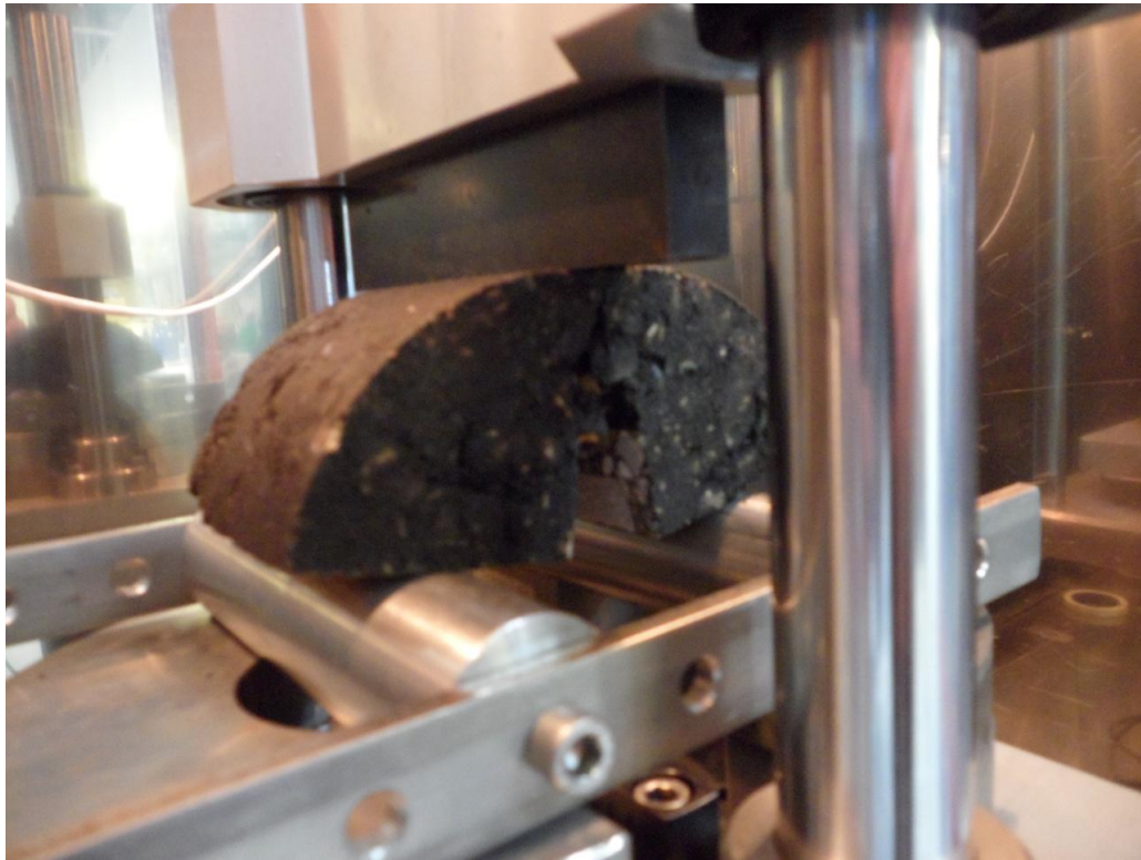
Figure 8: Crack Propagation during the Fracture Test.
