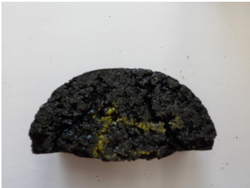
Figure (23): Failed SCB Specimen.
