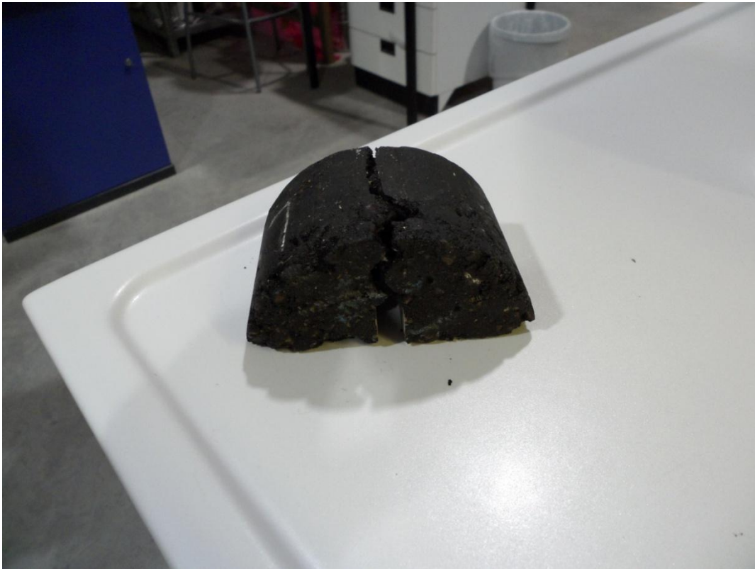
Figure 26: Failed SCNB Specimen.
