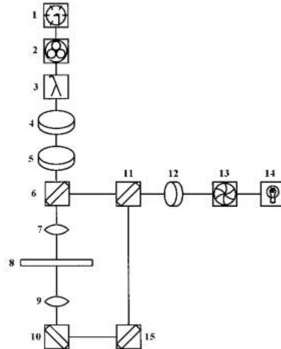
**Figure 1.** Optical plan showing photomultiplier (1), stray-light filter (2), grating monochromator (3), analyzer (4), tilting compensator (5), beam splitter (6), objective (7), sample stage (8), substage condenser (9), fixed mirror (10), slide-in mirror (11), polarizer (12), solenoid shutter (13), halogen illuminator (14) and fixed mirror (15).
