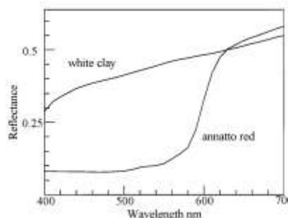
**Figure 4.** Fiber-optic reflectance spectra of annatto red on the white clay background of an Amazonian zunidor.
