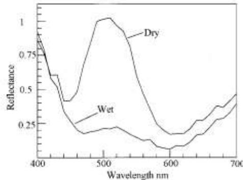
**Figure 8.** Iridescent blue on barbules of a peacock feather extinguished by wetting.
