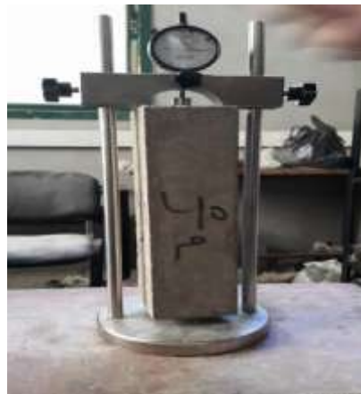
Figure 4: Specimen in length comparator
