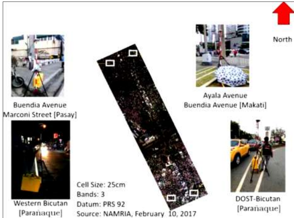
Figure 3: Orthophoto map and locations of 4 GCPs
