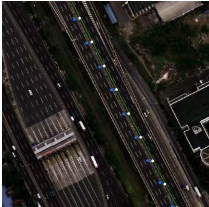
Figure 6: Deviations of points from the centerline (green line). White dots are data from MADOCA-PPP and blue dots are data from SPP. Here, the car is traveling northbound but the blue dots are already located on the southbound lane (beyond the center island).
