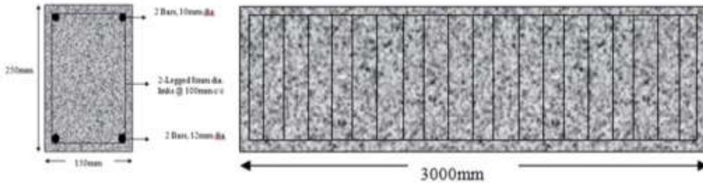
**Fig. 1 Reinforcement Details of the Beam Specimen**
