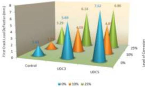
Fig.12 Effect of GFRP on Deflection at First Crack Deflection
