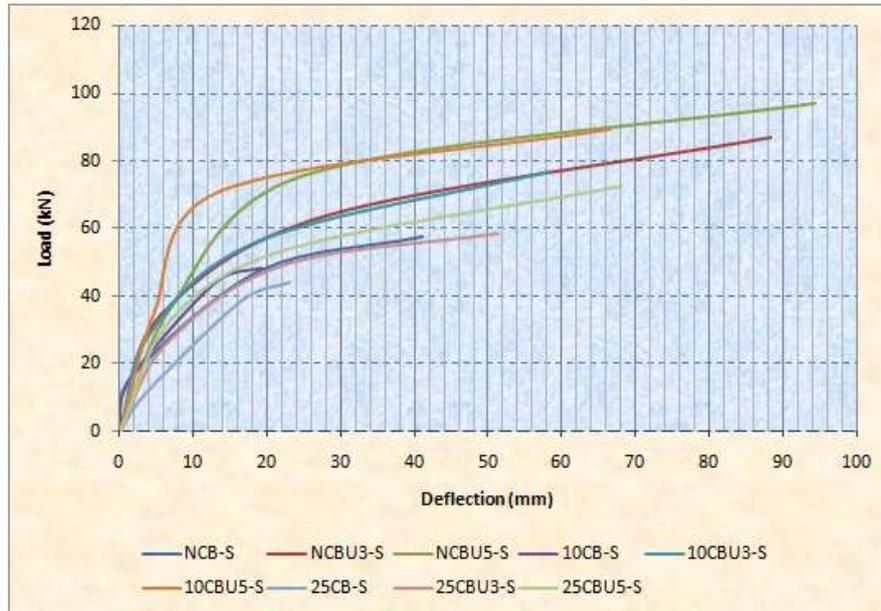
**Fig. 19 Load-Deflection Response of Control and Corroded - Strengthened HPC Beams**
