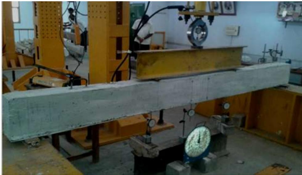
**Fig.8 Test Set-up for Static Loading**
