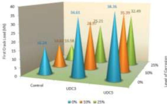
**Fig.9 Effect of GFRP on First Crack Load**
