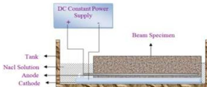
**Fig.7 Schematic of Accelerated Corrosion Set-up**
