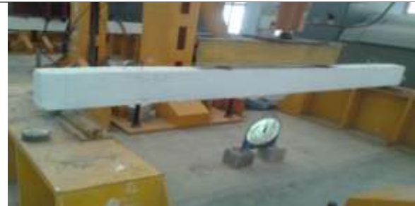
Figure 6: Experimental Test Set-up for Cyclic Loading
