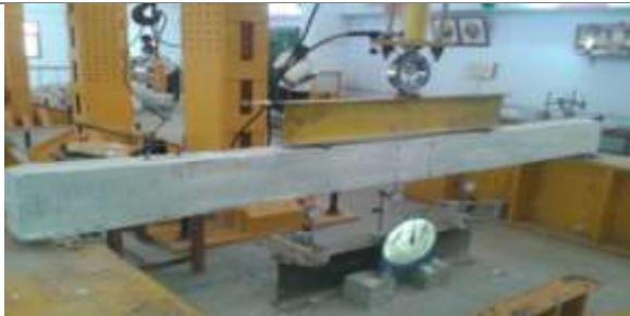
Figure 5: Experimental Test Set-up for Static Loading
