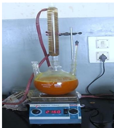
Figure 4: Experimental set for Esterification and Transesterification
