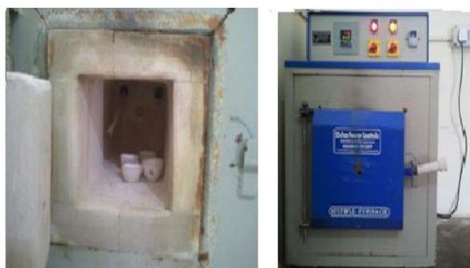
Figure 6: Photograph of catalyst preparation and the Muffle Furnace
