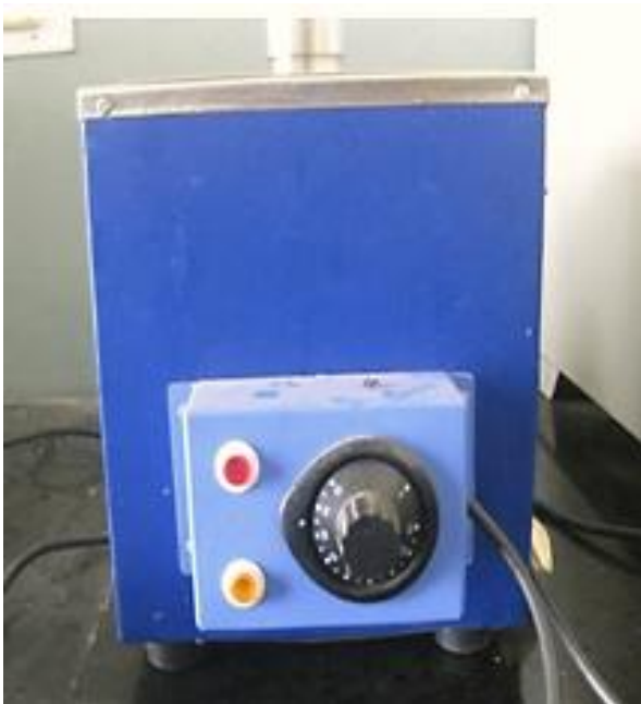
Figure 15: Copper strip corrosion instrument
