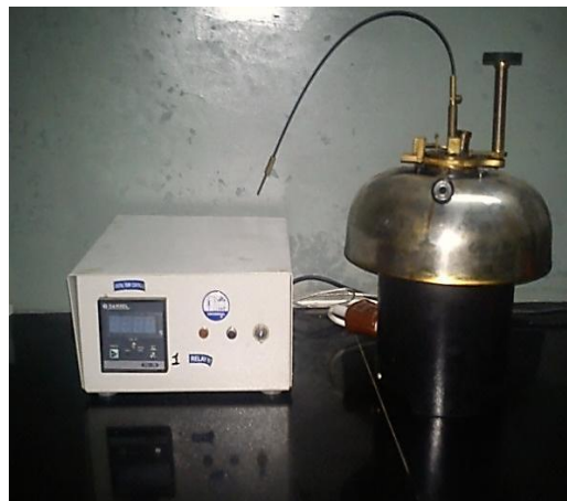
Figure 11: Photograph of Pensky Martin Flash point instrument
