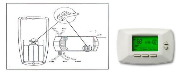
Figure-4: Thermostatic Ceiling Fan and Light Remote Control System
