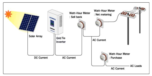
Figure-5 : Grid Tie Solar Power System
