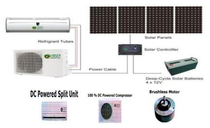
Figure-1: D.C. Powered Solar Air conditioner System
