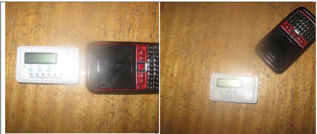
Fig.1 Set-up for measurement with DUT and Radiation Meter at different angles
