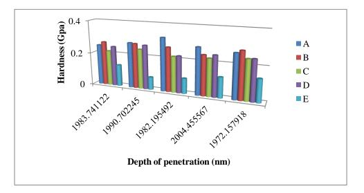
Figure 4: A graph of hardness against depth of penetration of five cattle horn samples
