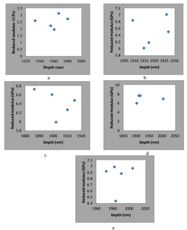
Figure 6: Reduced modulus against depth of penetration for the five cattle horn samples individually
