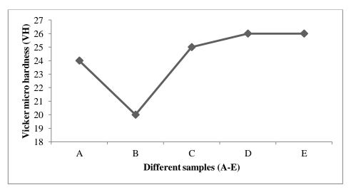
Figure 5: Variations of Vickers micro hardness with different samples
