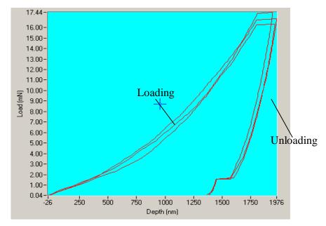
Figure 2: Loading and unloading curve for the cattle horn obtained using Berkovich indenter during loading and unloading
