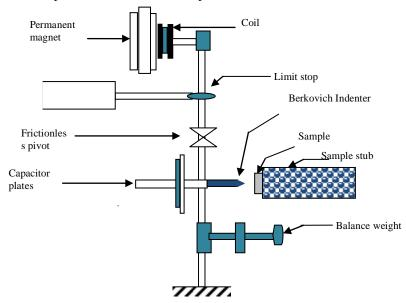
Figure 1: Experimental set-up for nanoindentation test
