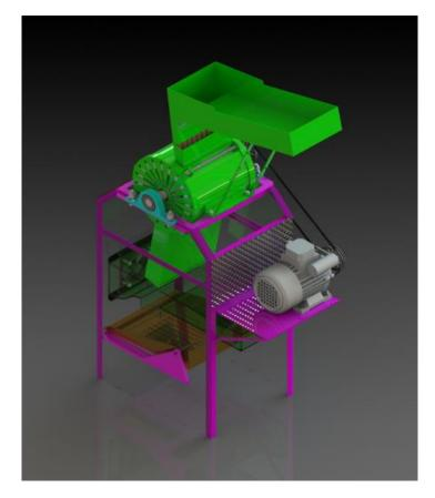
**Figure 2** Machine Assembly (3D) Nomenclature of the New Machine Design
