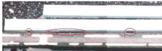
Figure 5: Die1 (bottom die) voids
