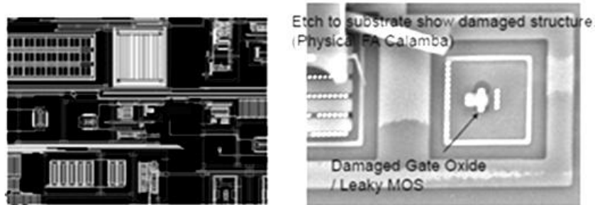
Figure 6: Damage gate oxide with plasma process
