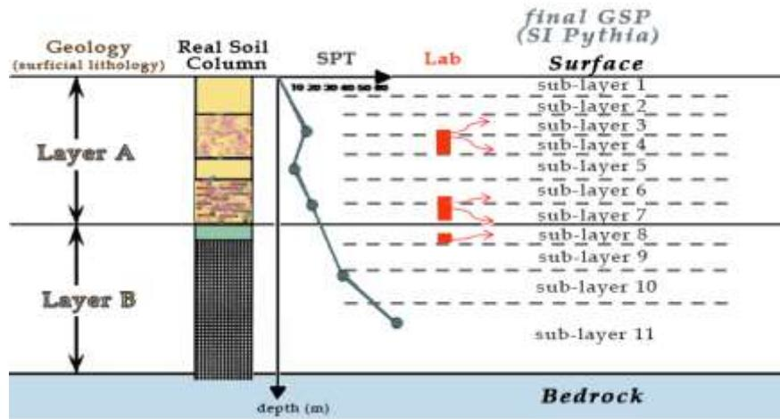
**Figure 4:** An Example on How a Geotechnical Soil Profile (GSP) is Created by SI
