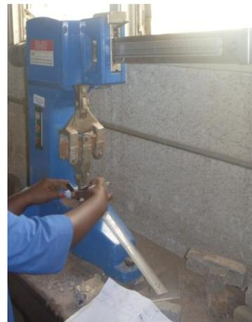
Figure. 2b: Flexural Machine
