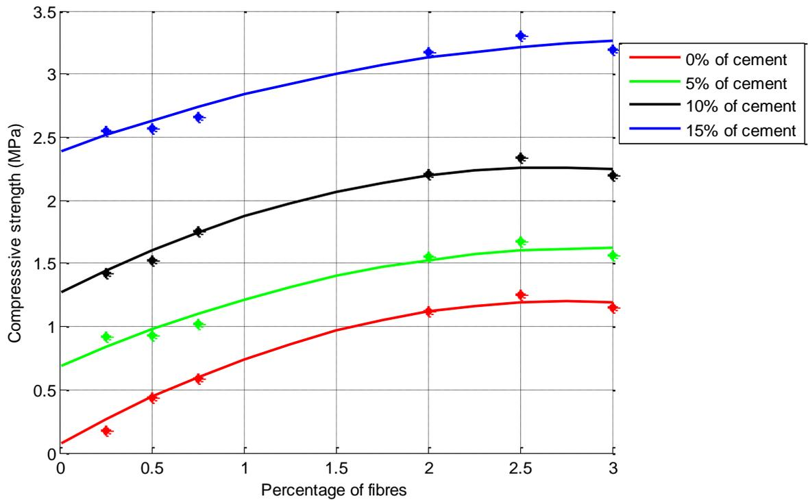
**Figure 5:** Average Compressive strength vs % spikelet fibres for 7 days of curing
