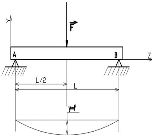
Figure. 2a: 3 point bending test
