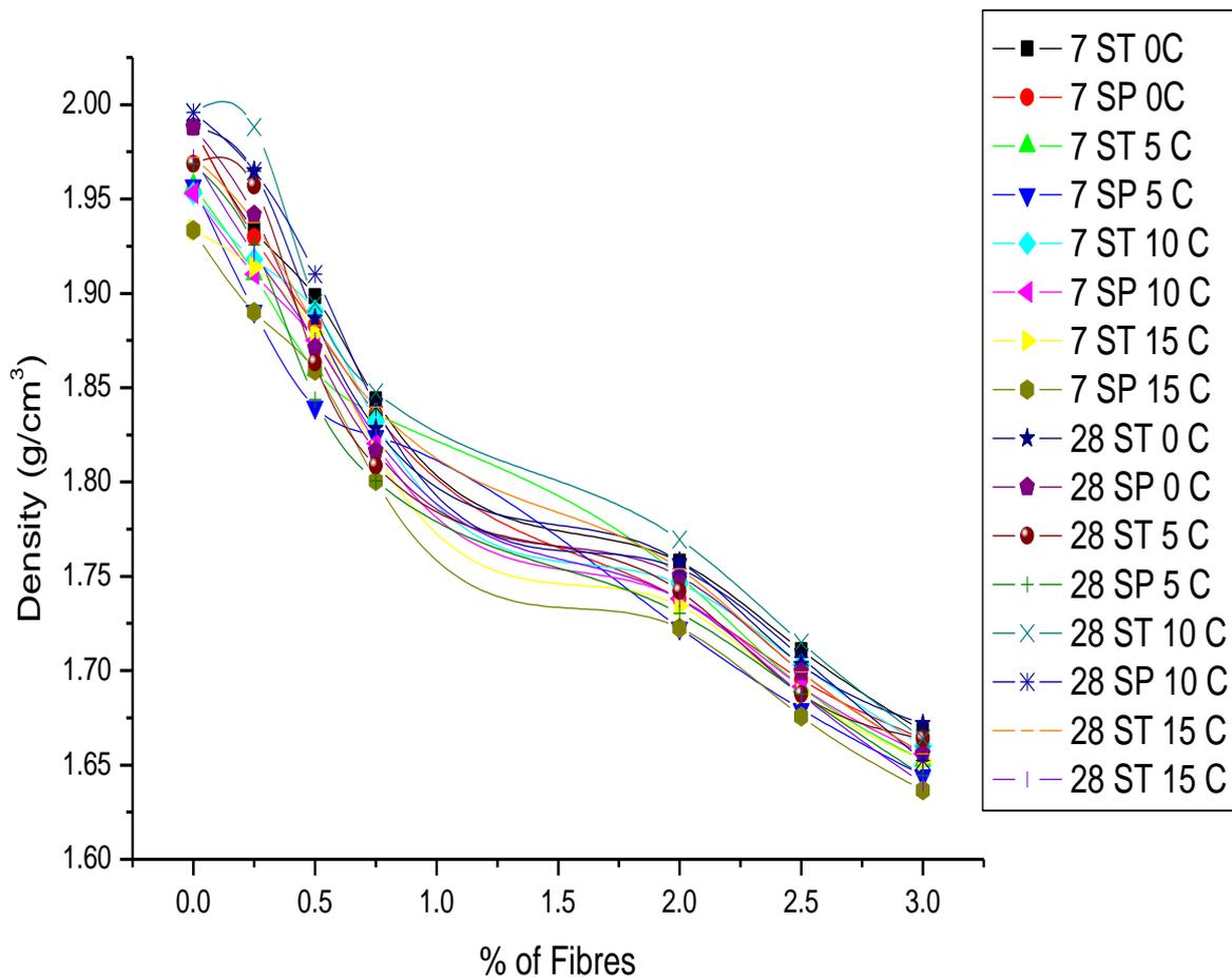
Figure 3: Densities of stabilized reinforced composites
