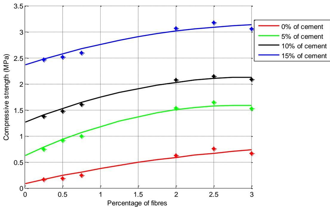
Figure 4: Average Compressive strength vs % Stalk fibres for 7 days of curing
