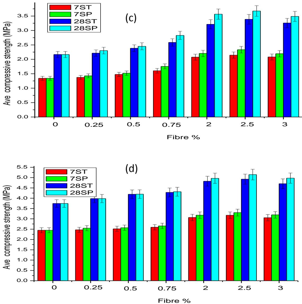
Figure6: Compressive error bar for 7 and 28 days with a) 0% cement b) 5% cement c) 10% cement d) 15% cement
