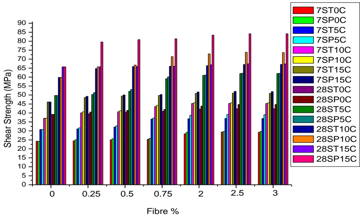
Figure 8: The Shear Strength of composites
