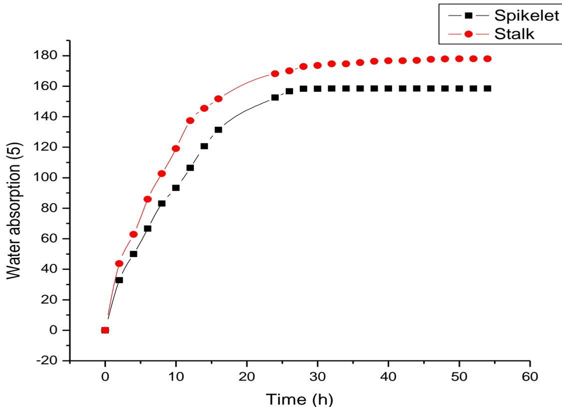
Figure 9: Water absorption of Stalk
