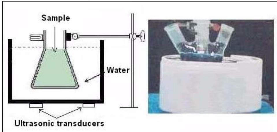
Figure 4 - Laboratory ultrasonic bath.
