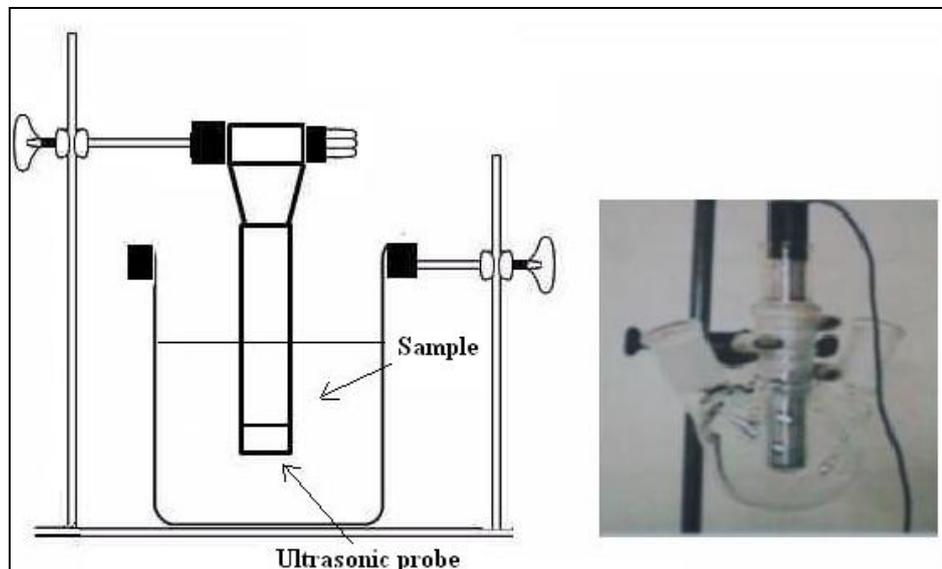
Figure 5 – Ultrasonic laboratory Cell for direct placement in the sample.
