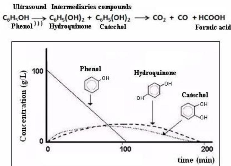
Figure 3 – Graph of the destruction of phenol by ultrasound.
