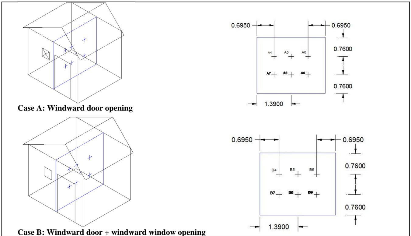
Figure 2: Defined points for Internal Pressure Measurements (2)
