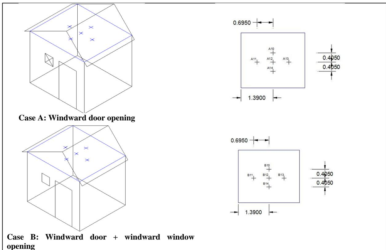
Figure 3: Defined points for Internal Pressure Measurements (3)
