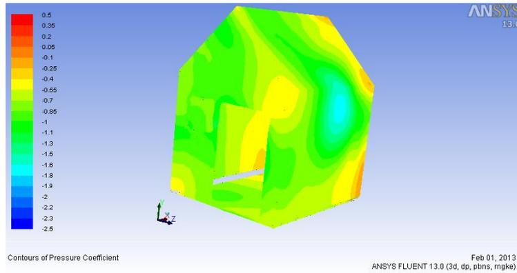
Figure 5: Contours of Pressure Coefficient (45° wind angle of attack)
