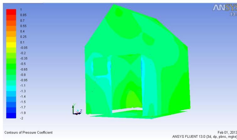
**Figure 4: Contours of Pressure Coefficient (90° wind angle of attack)**
