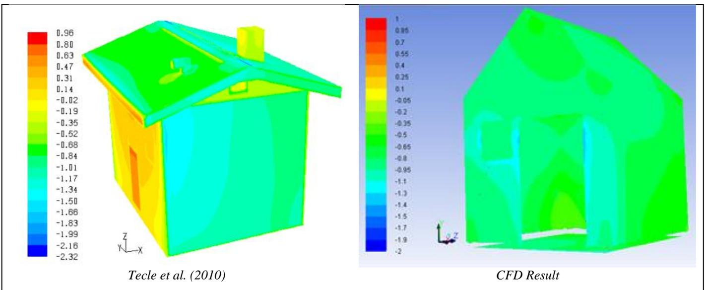
Figure 6a: External Pressure Coefficient for 90° wind angle of attack respectively in comparison with Teclé (2010)
