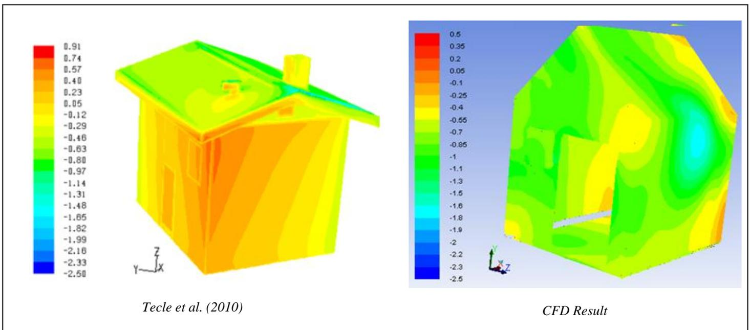
Figure 6b: External Pressure Coefficient for 45° wind angle of attack respectively in comparison with Teclé (2010)
