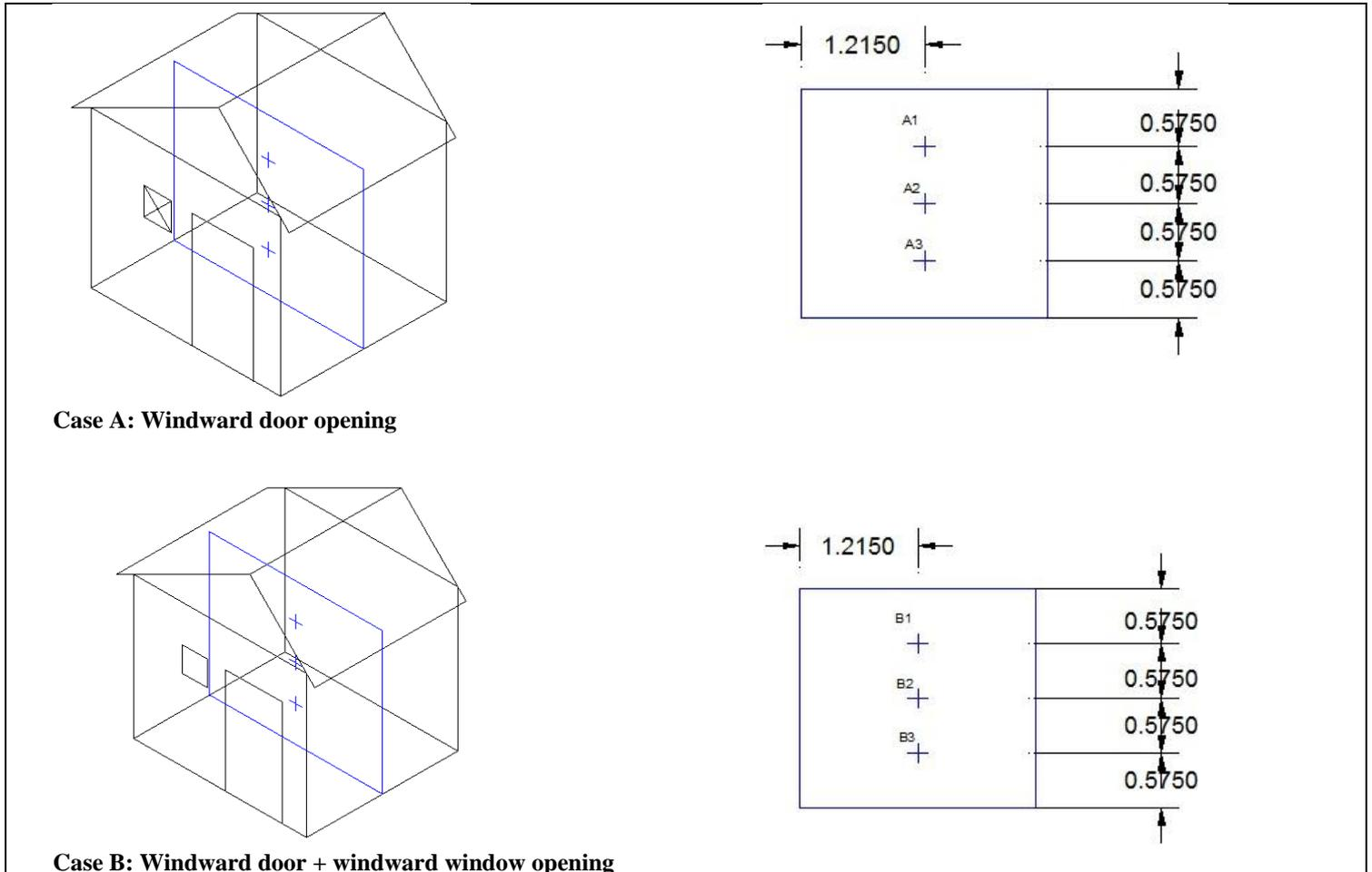
Figure 1: Defined points for Internal Pressure Measurements (1)
