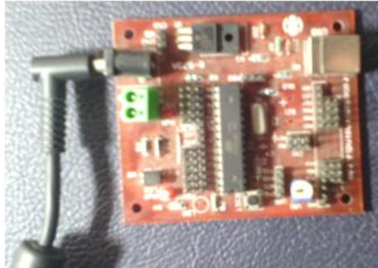
Figure 3.4: Atmega8 IC mounted in AVR development board
