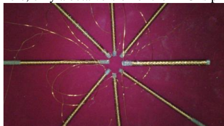
Figure 4.1: Field coils having eight pole paths
