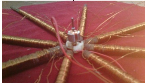
Figure 4.3: Field coils with armature winding
