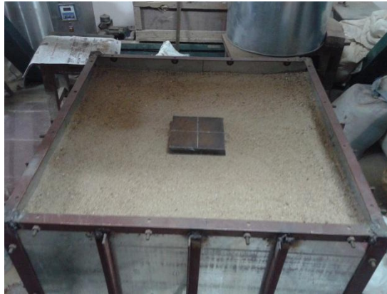
Figure 1: Sand Bed and Model Footing
