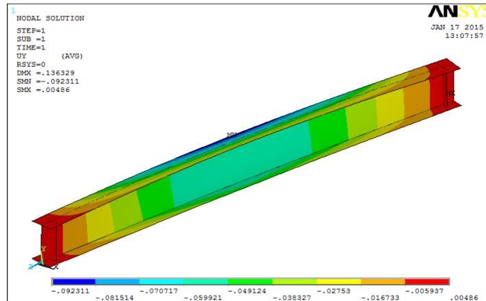
**Figure 6:** Contour plot of the vertical deflection of curved I-girder without stiffeners
