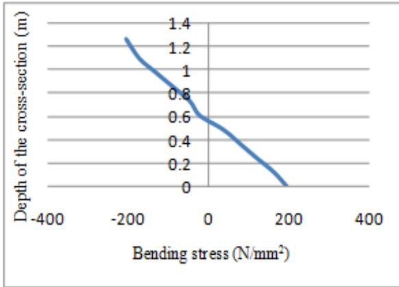
**Figure 9 :** Bending stress distribution of straight I-girder
