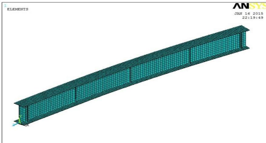
**Figure 4:** Meshed model of the curved I-girder with three intermediate stiffeners
