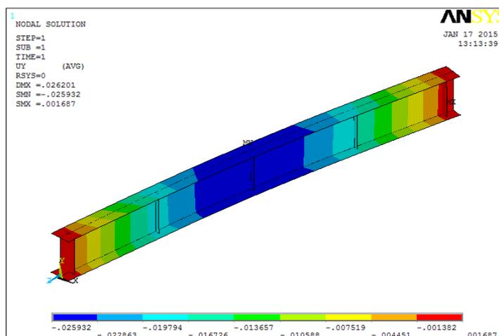
**Figure 8:** Contour plot of the vertical deflection of curved I-girder with three intermediate stiffeners
