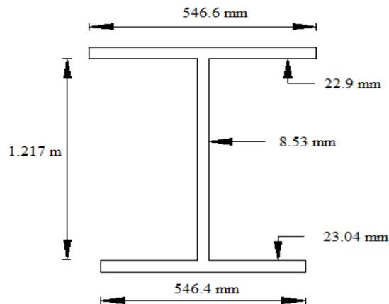
Figure 1: Cross-section of the I-girder
