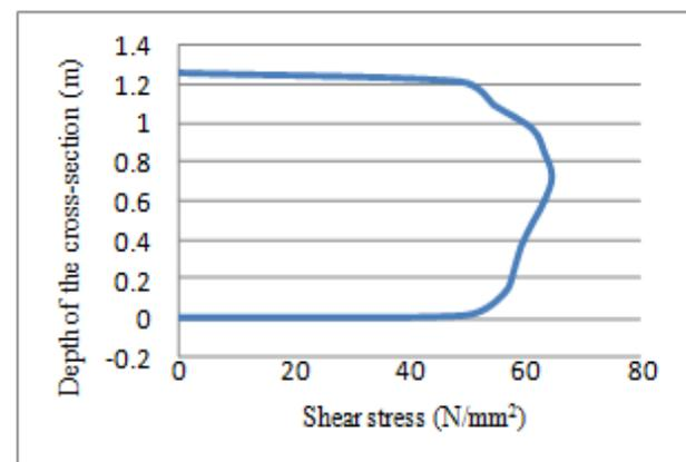
**Figure 14:** Shear stress distribution of curved I-girder with one intermediate stiffener
