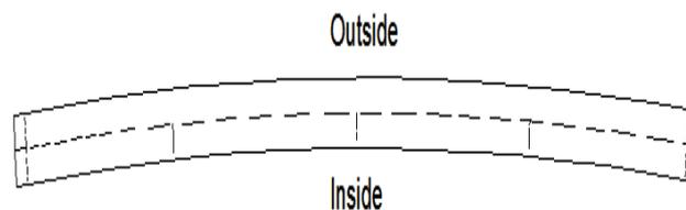
Figure 2: Top view of the curved I-girder
