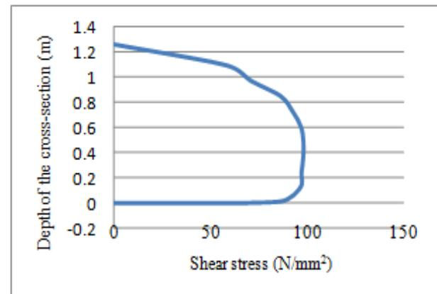
**Figure 12:** Shear stress distribution of curved I-girder without stiffeners
