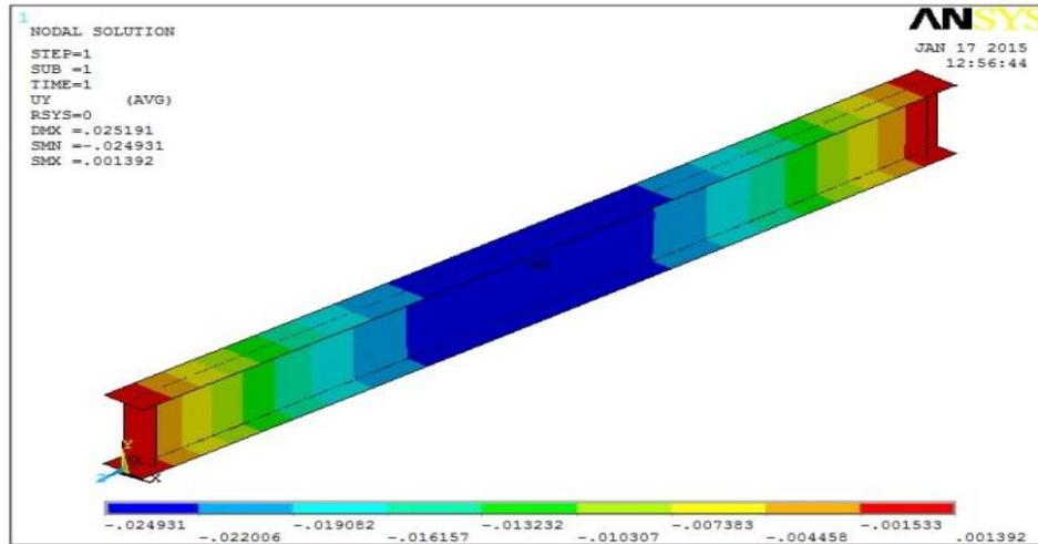
**Figure 5:** Contour plot of the vertical deflection of straight I-girder
