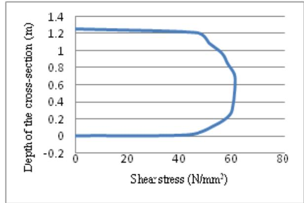
**Figure 10:** Shear stress distribution of straight I-girder
