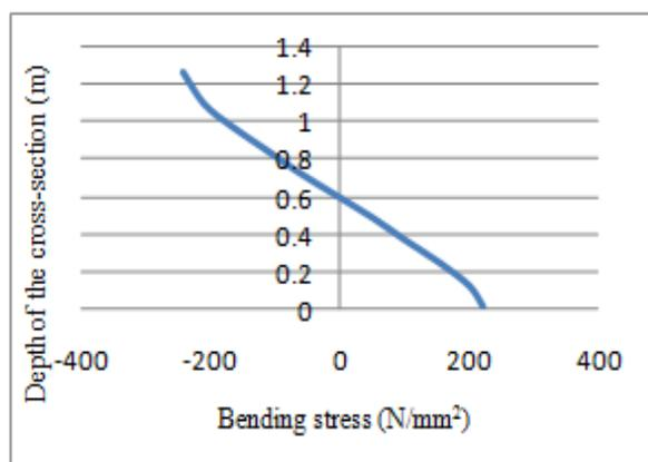
**Figure 13:** Bending stress distribution of curved I-girder with one intermediate stiffener
