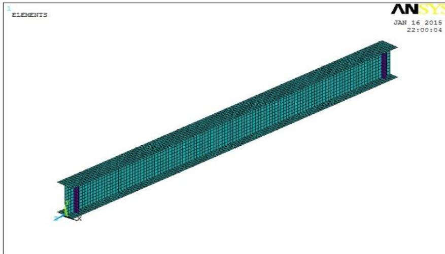
**Figure 3:** Meshed model of the straight I-girder
