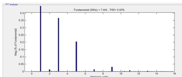
Figure 4: FFT Analysis of source current with single tuned filter
