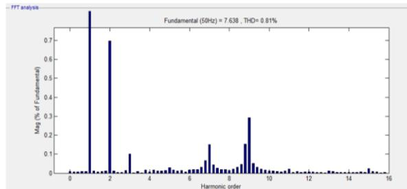
Figure 6: FFT Analysis of source current with C type filter
