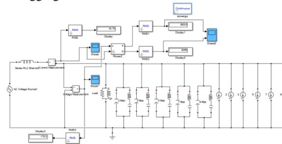
Figure 7: Simulink model of CCL filter
