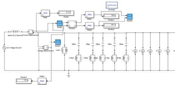
Figure 5: Simulink model of C type filter
