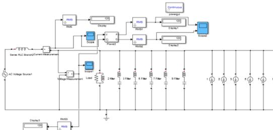
Figure 3: Simulink model of single tuned filter
