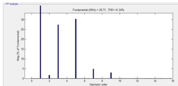
Figure 8: FFT Analysis of source current with CCL filter
