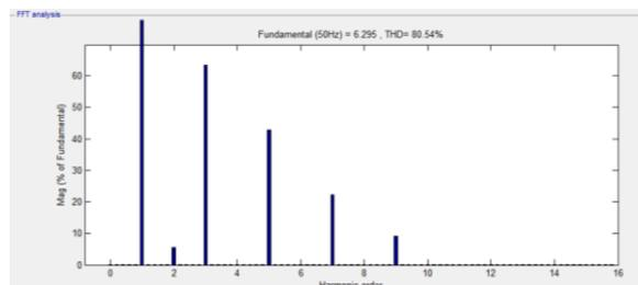
Figure 2: FFT Analysis without filter
