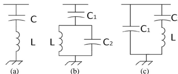
**Figure 1:** Different Filter Topologies (a) ST Filter (b) C Type Filter (c) CCL Filter [5]
