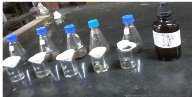
Figure 6: Filtration of sample
