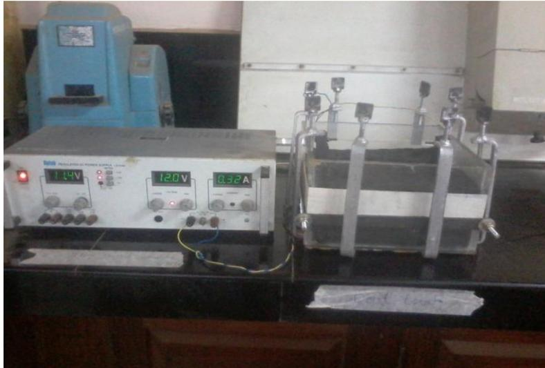
Figure 1: Experimental setup for electrochemical remediation
