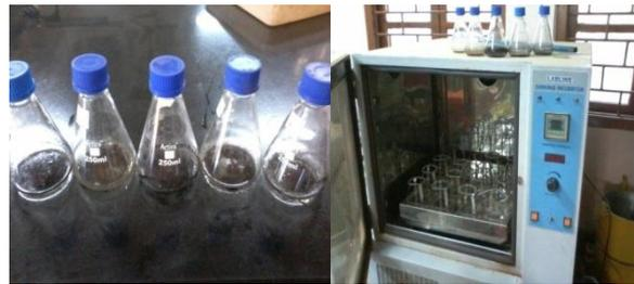
Figure 5: Soil+oil+hexane mixture and mechanical shaker
