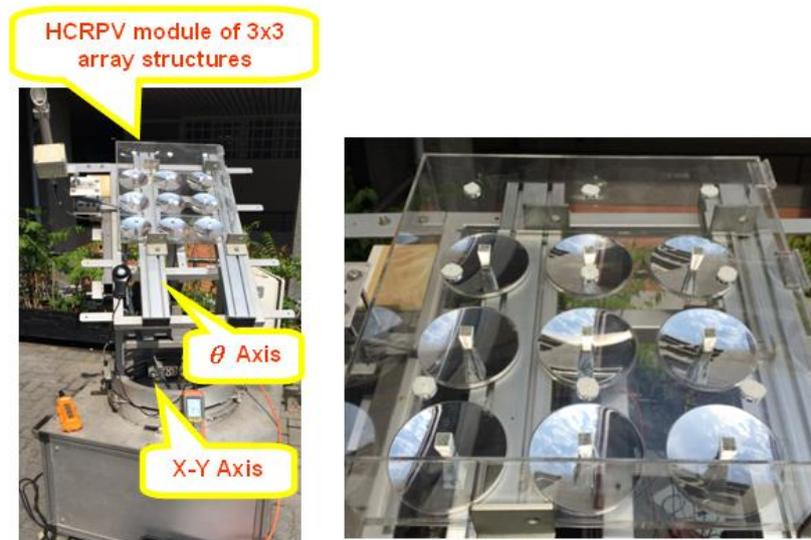
Figure 4 The fabricated HCRPV module with the light guide tube
