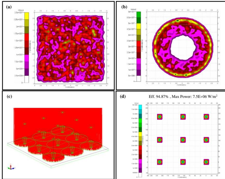
Figure 3 Configurations of designed structures and simulation results: (a) light spot diagram with the light guide tube and (b) light spot diagram without the light guide tube and (c) 3x3 array modules and (d) light spot diagram of 3x3 array modules.
