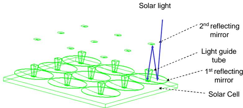
Figure 1 Configurations of designing HCRPV modules of 3x3 array structures with light guide tube
