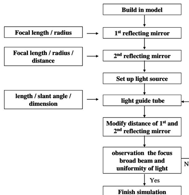
Figure 2 Flow chart of simulation procedure
