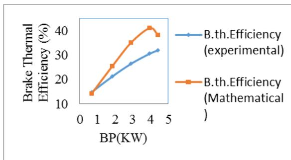
Figure9: Variation of Brake Thermal Efficiency w.r.t Load
