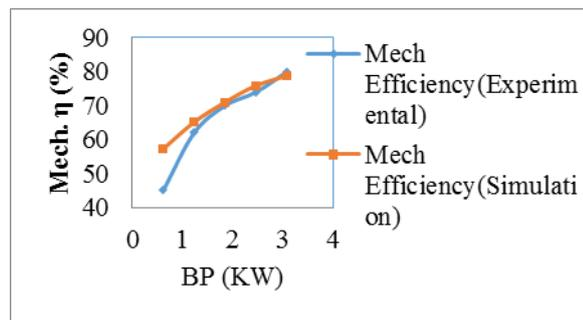
Figure4: Variation of Mechanical Efficiency w.r.t BP
