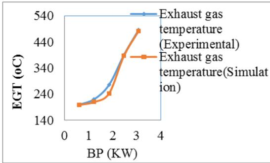
Figure5: Variation of Exhaust Gas temp w.r.t BP
