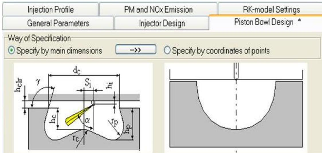
Figure1: Hemispherical Piston Bowl Modelled with Diesel
