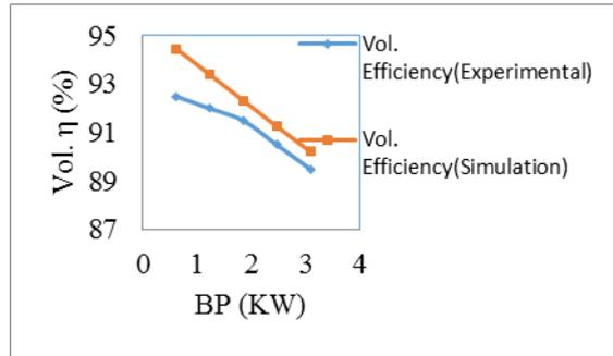
Figure6: Variation of Volumetric Efficiency w.r.t BP
