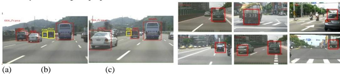
Figure 9: (a) (b) The vehicle identification process, (c) Examples of detection results.
