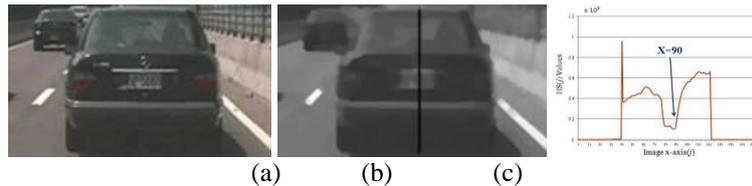
Figure 6: (a) Original image, (b) symmetry measurement, (c) symmetry measurement result with local minimum at  $x=90$ .
