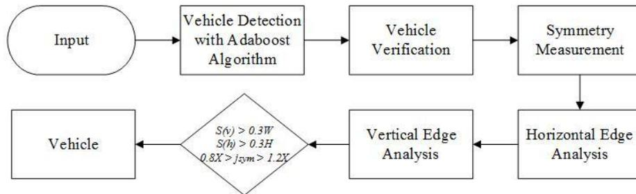
Figure 1: The vehicle detection system flowchart.
