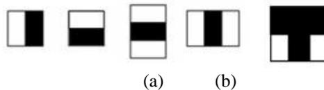
Figure 2: The proposed AdaBoost classification features: (a) Haar-like feature and (b) the proposed car-like feature.
