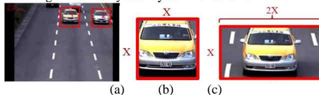
Figure 5: Vehicle Candidate Area Selection: (a) Vehicle Detection Results, (b) Original Vehicle Candidate, (c) Vehicle Candidate Symmetry Measurement Area.
