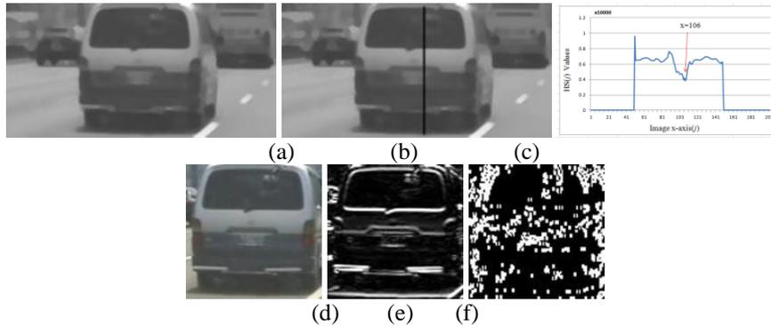
Figure 10: The vehicle verification for a hit case: (a) median filtering result of vehicle candidate image, (b) (c) symmetry measurement result, (d) vehicle candidate region, (e) horizontal edge detection result, (f) vertical edge detection result.
