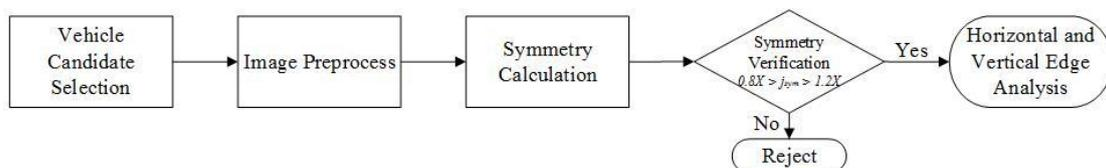
Figure 4: The symmetry measurement flowchart.
