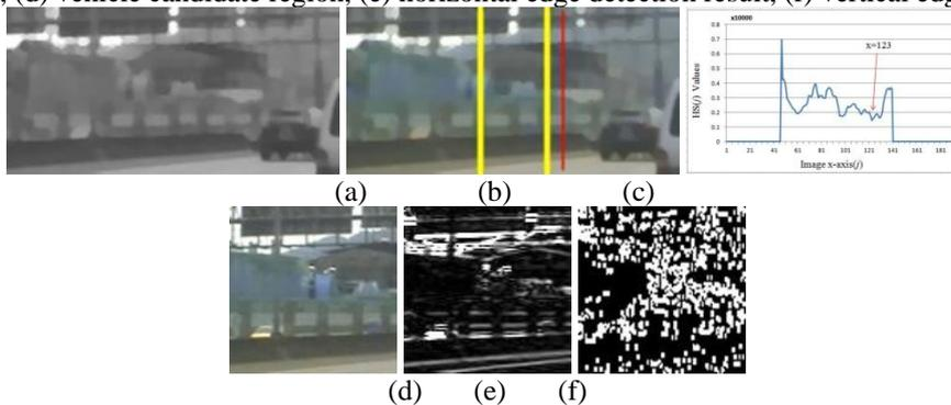
Figure 11: The vehicle verification for a false case: (a) median filtering result of vehicle candidate image, (b) (c) symmetry measurement result, (d) vehicle candidate region, (e) horizontal edge detection result, (f) vertical edge detection result.
