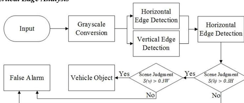
Figure 7: The horizontal and vertical edge analysis flowchart.
