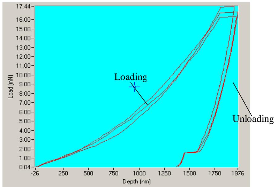
**Figure 2:** Loading and unloading curve for the cattle horn obtained using Berkovich indenter during loading and unloading
