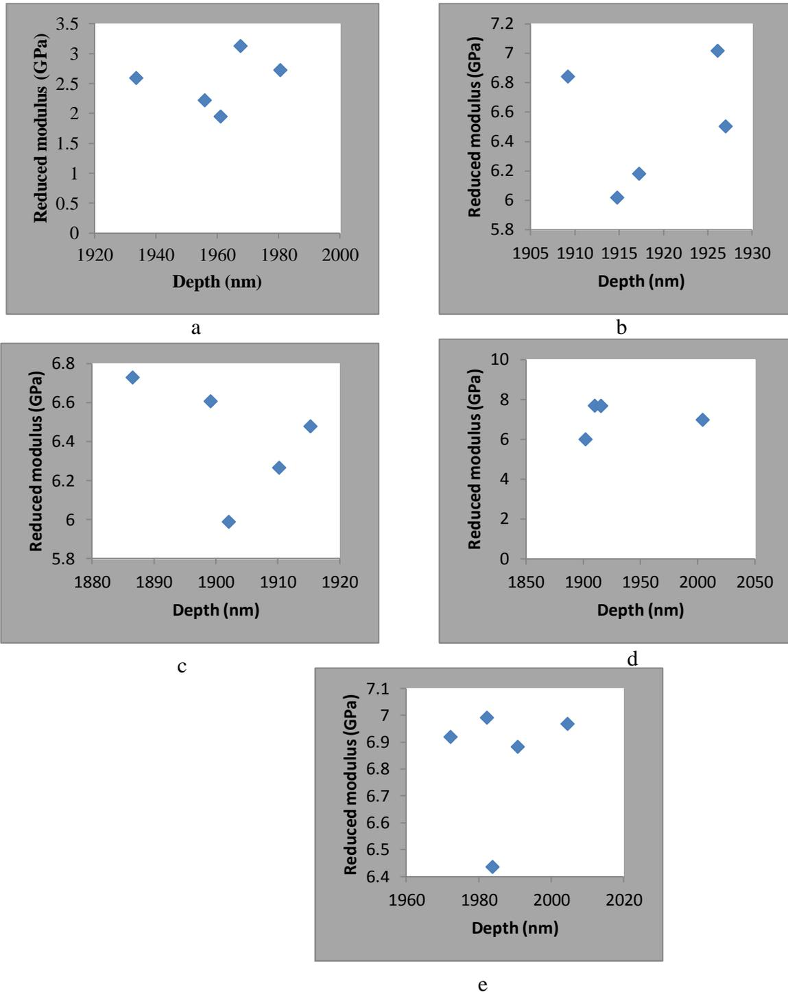
**Figure 6:** Reduced modulus against depth of penetration for the five cattle horn samples individually
