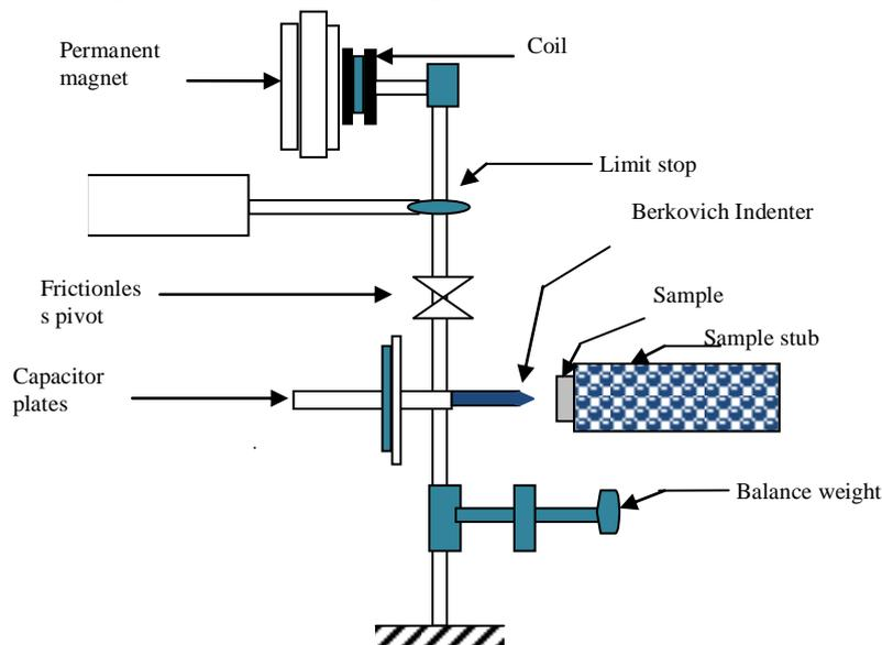
Figure 1: Experimental set-up for nanoindentation test
