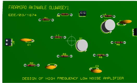
Fig 8: PCB Board layout for LNA design
