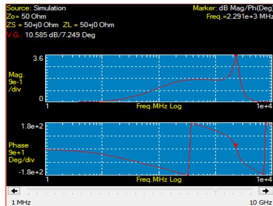
Fig 4: Multisim simulation of LNA Design Gain
