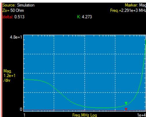
Fig 3: Multisim simulation of LNA Design stability
