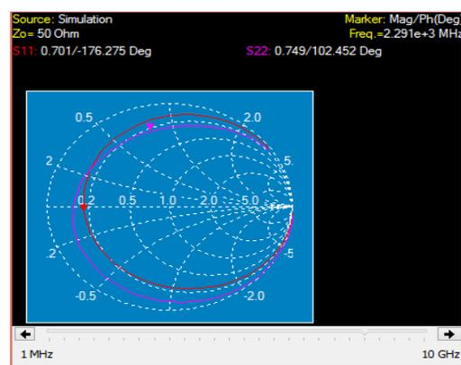
Fig 6: Multisim simulation of LNA Design S-Parameter
