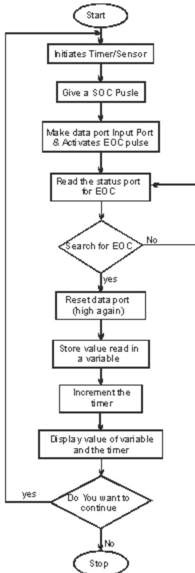
**Figure 3: Flow Chart for Data Acquisition**
