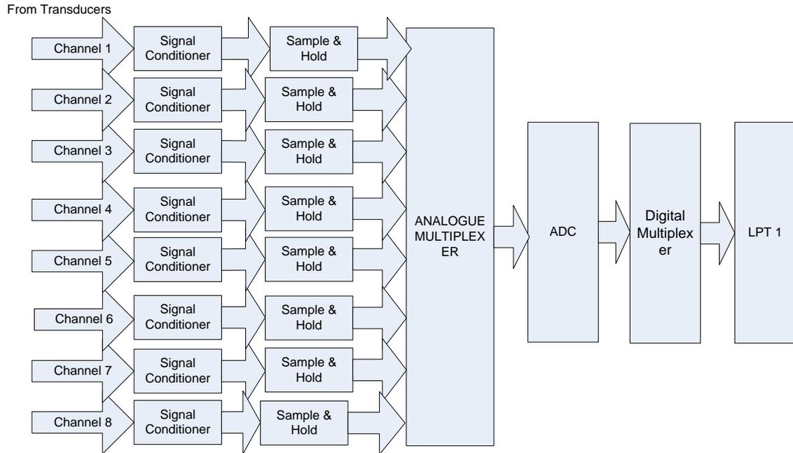
Figure 1. Block Diagram of Eight Channel Data Acquisition System
