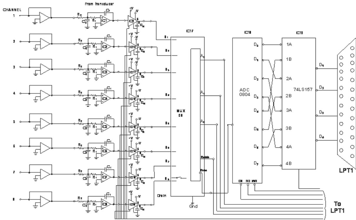
Figure 2: Circuit Diagram of Data Acquisition System
