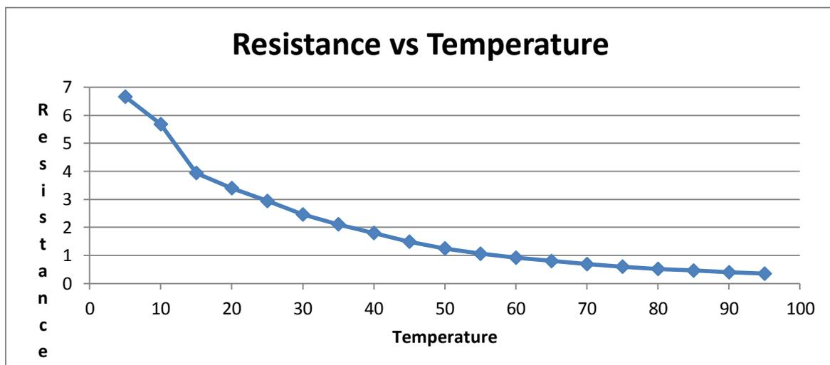
Figure 4 Graph of Resistance vs Temperature for TH1 Thermistor
