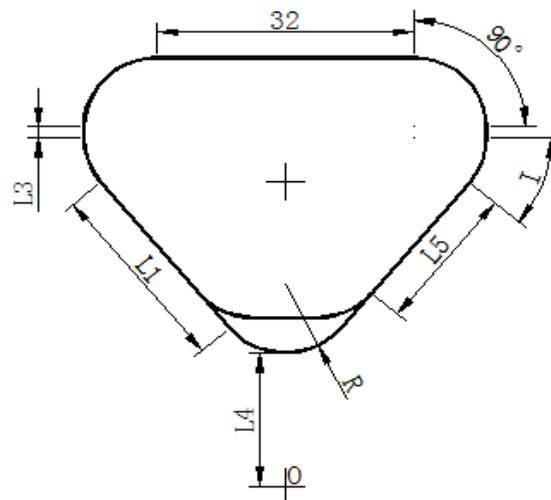
(b) Typical structure of mold cavity with a slope
