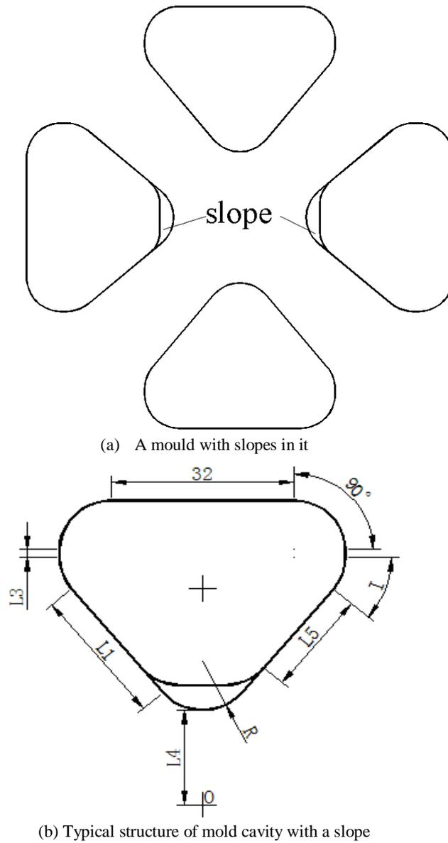
**Figure 11:** Mould cavity with slopes
