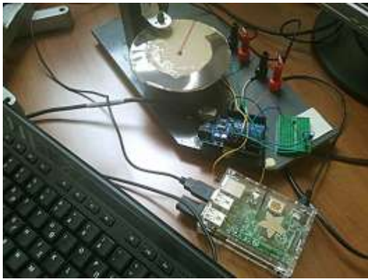
Figure 4: The experimental apparatus. One can observe the Raspberry Pi in the foreground, whereas the Arduino controller placed near the rotating disk.
