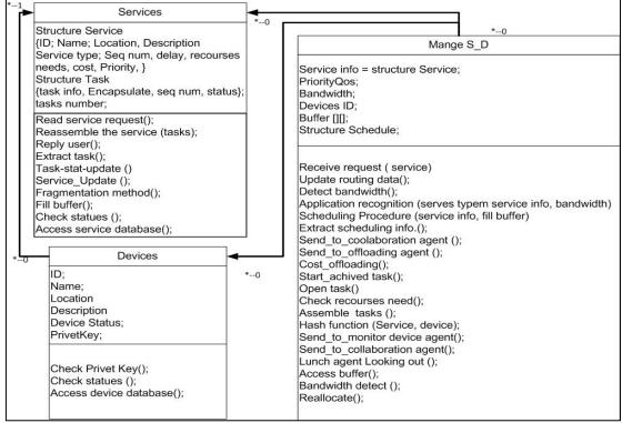
Figure 6: Class Diagram
