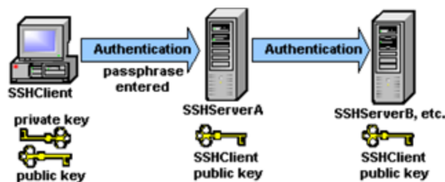
Figure7: Agent Forwarding passes authentication from the first SSH connection to the next, re-authenticating each time.
