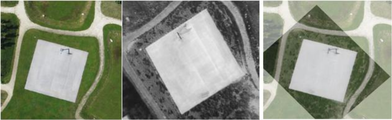
Figure 1 Image pair from dataset and images registered using Homograph estimated
