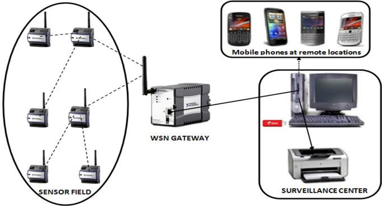
Figure 3.2 – Architecture of the FMDS
