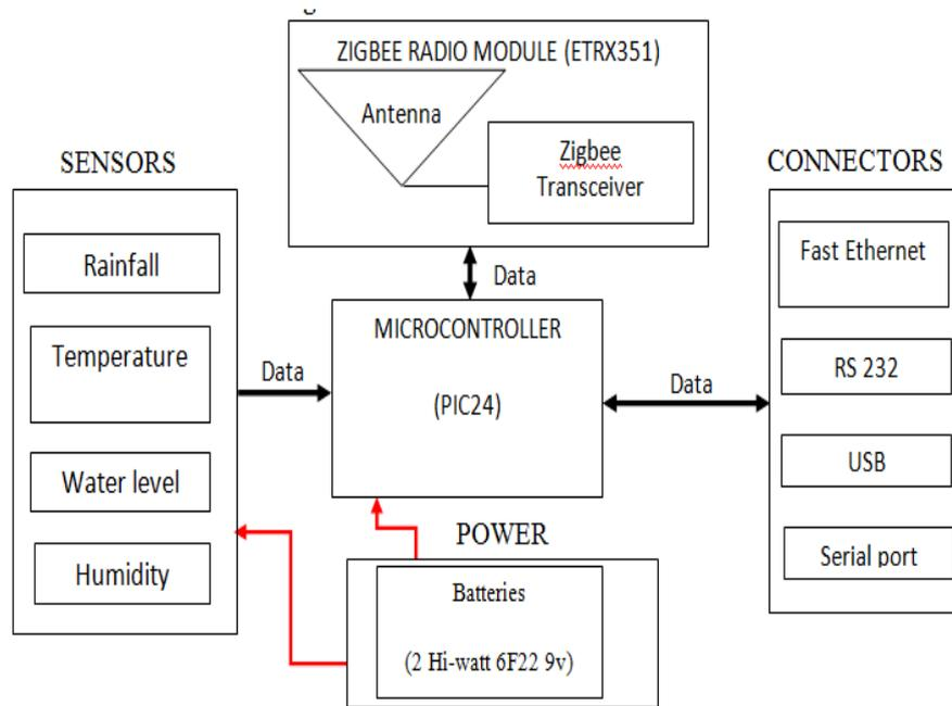
Figure 3.1 – Hardware design block diagram
