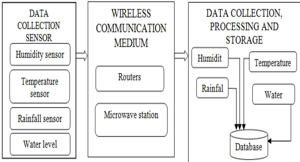
Figure 3.3 – Block diagram of the proposed FMDS
