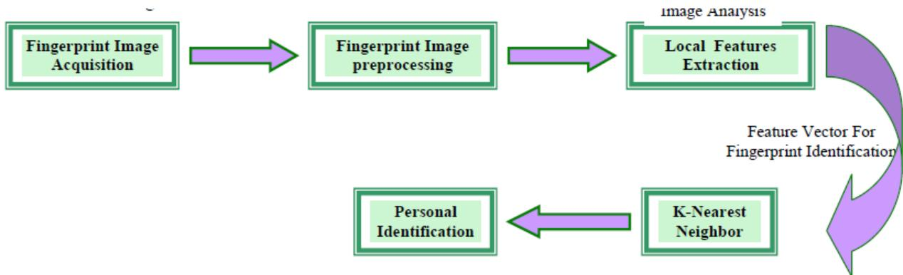
**Figure 5:** The Block Diagram of the Proposed System.
