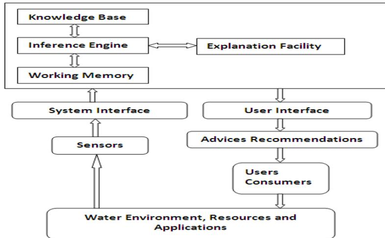
Figure 2: Structure of proposed expert system
