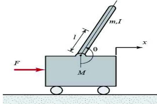
**Figure 1:** Schematic diagram of cart and inverted pendulum
