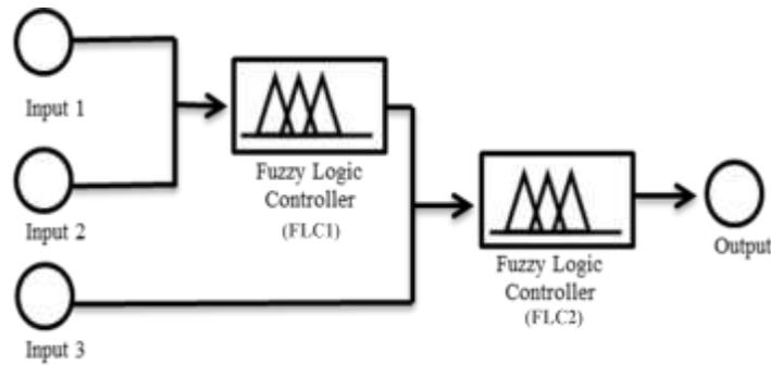
Figure 3: Structure of fuzzy Logic controllers FL
