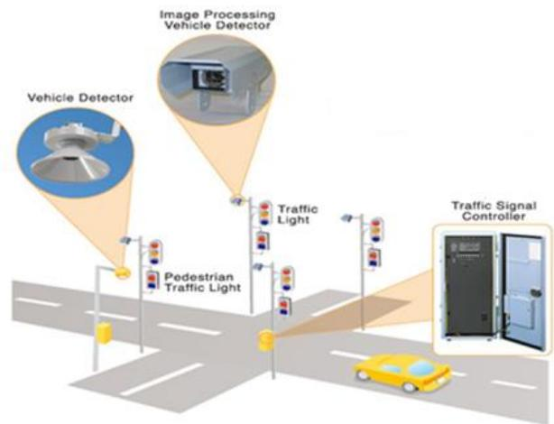
**Figure 4** Intelligent Traffic Control System
