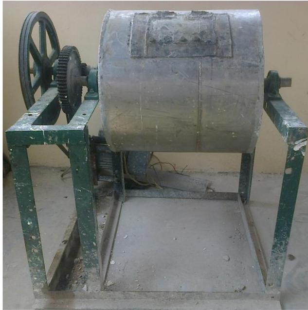
Figure 2: Prototype Design of Ball mill
