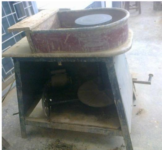
Figure: 3 Prototype Design of Electric Potters Wheel
