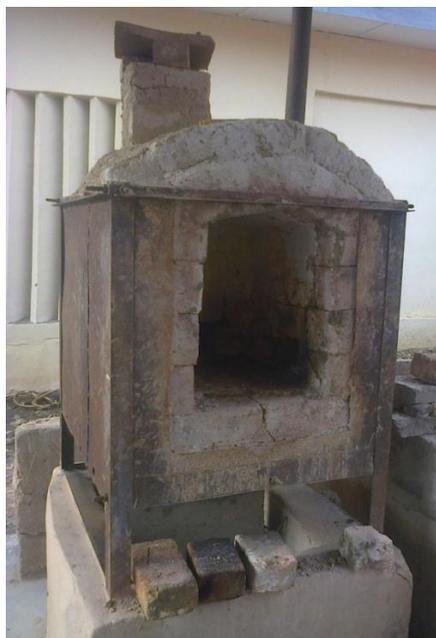
Figure 2: Prototype Design of Test Kiln
