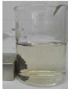
Figure 2. Magnetic separation of nanoparticles coated with mucilage into grains
