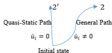
Figure 1. Different feasible paths for applying the same amount of energy
