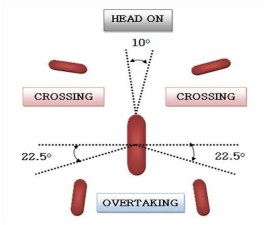
Fig. 7 Encounter types according to COLREG
