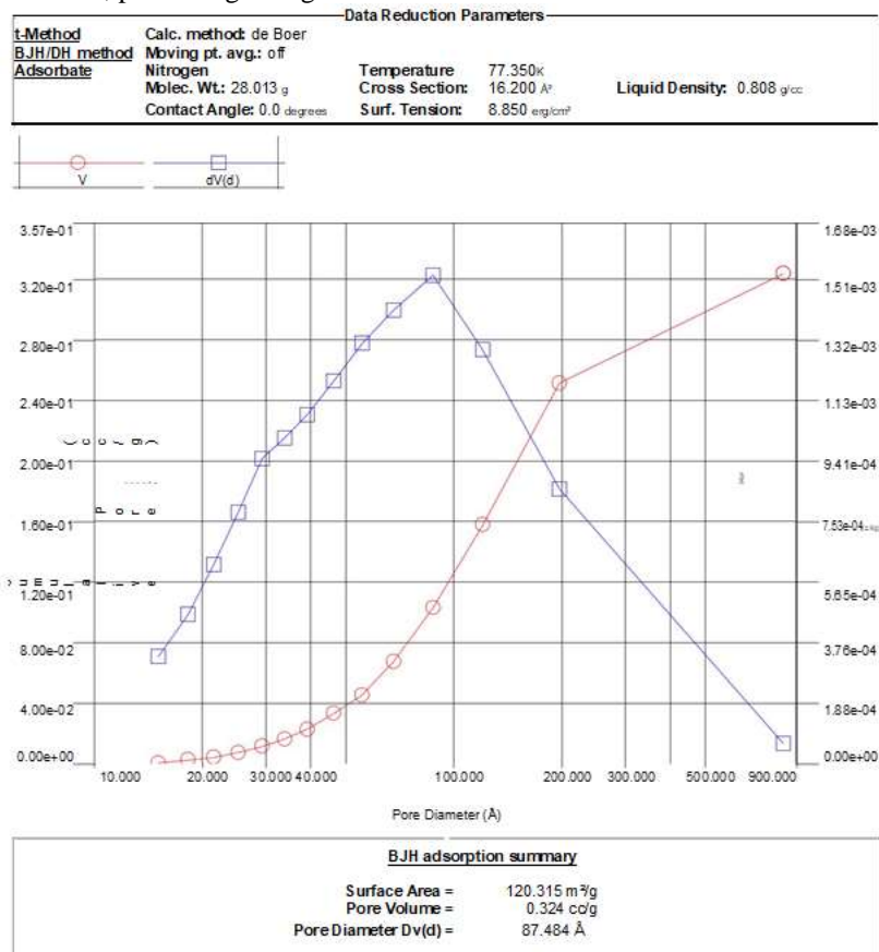
Figure 5: Chart of pore diameter and specific surface area of optimal VNBC sample
