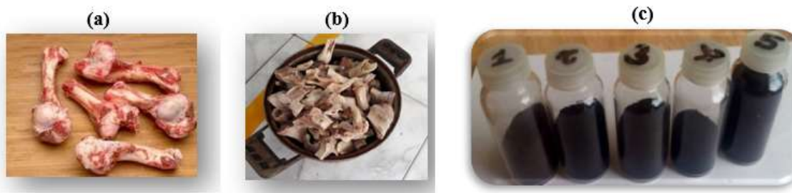
Figure 2: The images of VNBC synthesis process in laboratory. It is denoted that Figure (a) as bovine bones collected from cow slaughterhouse, Figure (b) as bovine bones cleaned, and Figure (c) as bovine bones synthesized to VNBC, respectively.
