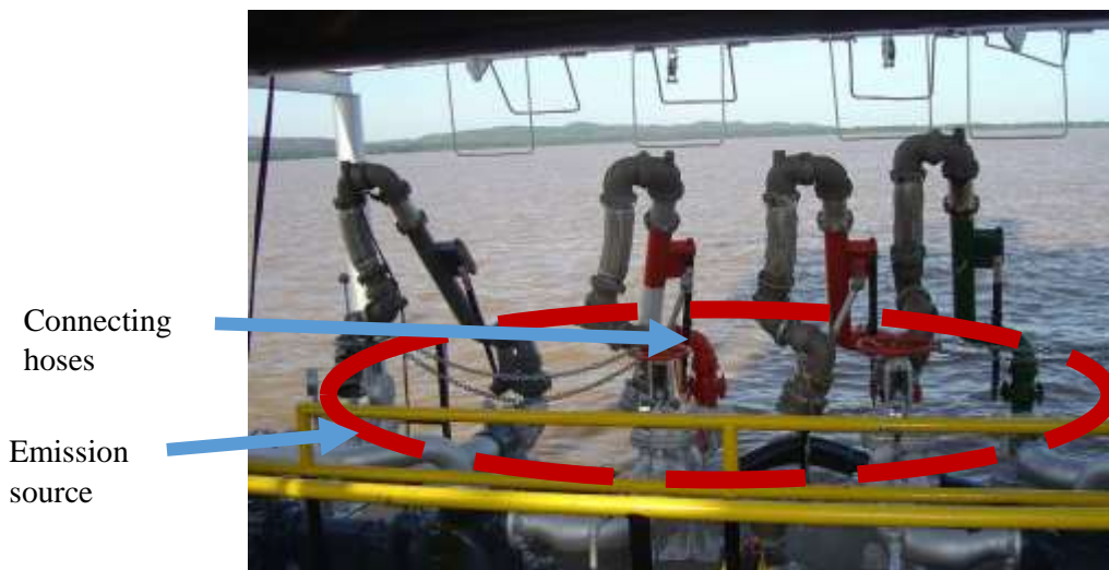
Figure 5. loading barge operation
